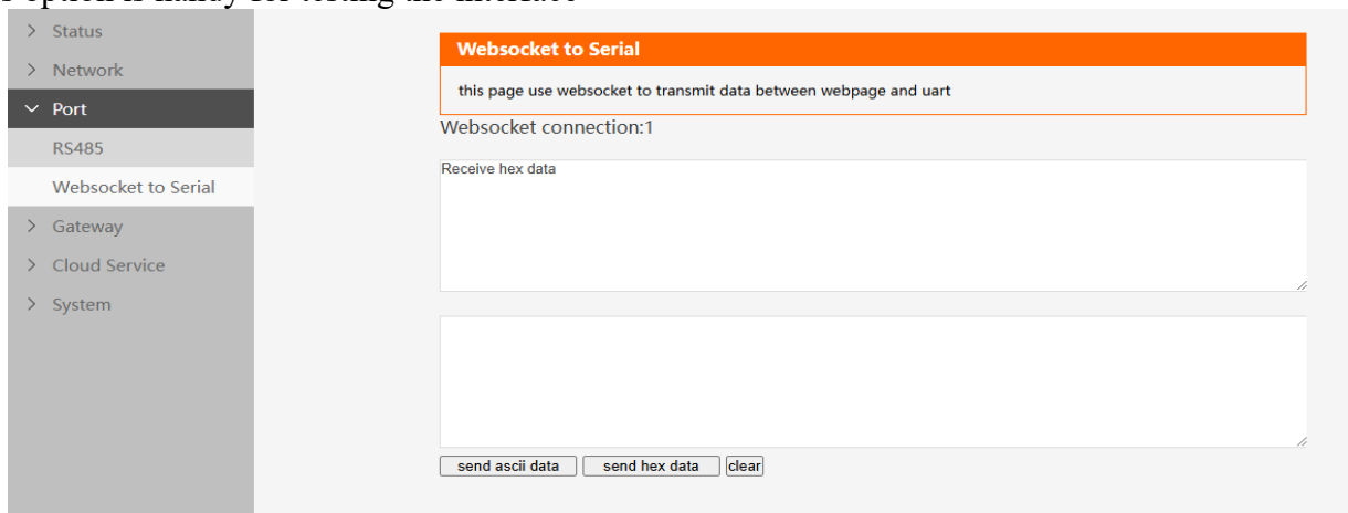
Fig 6 Send and receive data using webpage
